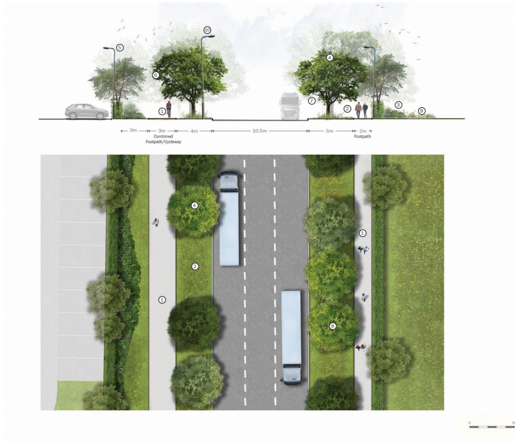
Fig 17. Typical Sections through Internal Distributor Roads (sheet 1 of 2) – Numbers relate to Design Code Text below
